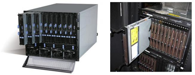
High-Density Servers are a new type of server developed in response to the high-density configuration of data centers. The more well-known product is the Intel-based x86 high-density server System x iDataPlex launched by IBM in 2008, this half-deep 2-socket server can accommodate two servers in a 2U chassis. However, two 2U chassis can be placed in the 2U cabinet space. On average, each 1U height density can also host two servers.
