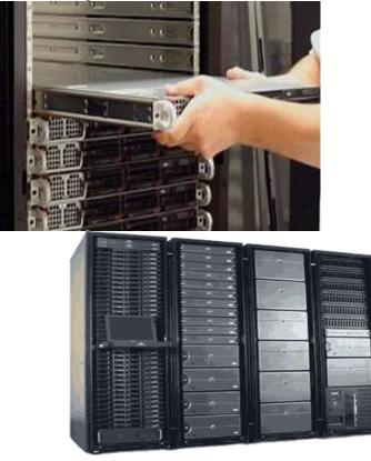
Blade servers It is a single-board server proposed by RLX in 2001. A blade server consists of a complete chassis that provides functions such as power supply, fan cooling, and network communication in a centralized manner. Multiple system motherboards can be inserted into the chassis, therefore they are called blade servers. Currently, there is no unified standard for the chassis' appearance and the number of servers that can be accommodated. It is specially designed for special
